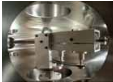
Transfer Arm inside RDC Chamber
